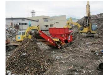
Separate process of large quantities of garbage generated by the Tohoku Earthquake using wood crushers
